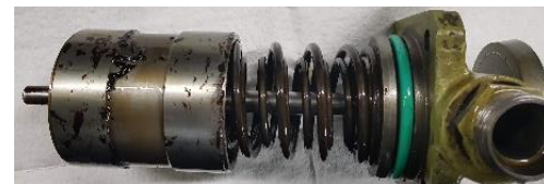
Figure 6: A Failed valve coated with varnish deposits.
