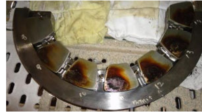
Figure 5: Deposit formation on a bearing, showing surface damage at its highest load zone.
