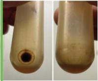
ULTRACENTRIFUGE WITHOUT DECON (LEFT) AND AFTER DECON (RIGHT):
