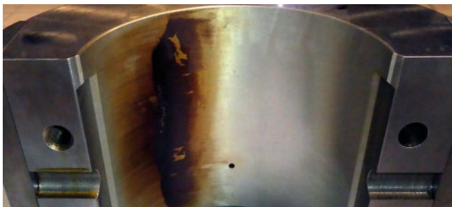
View into a pinion bearing: Before ...
