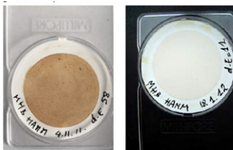
Fig.6: MPC patch tests from MVA Hamm Turbine in 2011 (left) and after 1 year service (right)
