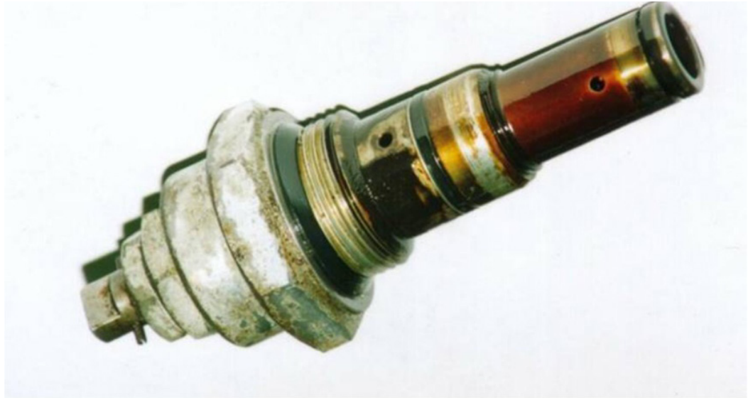
Figure 1: A small layer of varnish deposit due to hydraulic oil oxidation can lead to servo-valve sticking, accelerated wear and malfunction. (Source: A. Sasaki)
