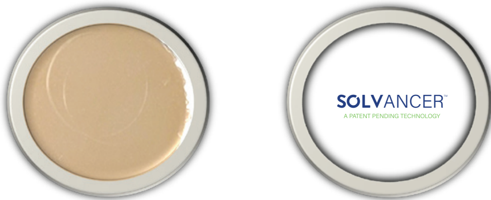
Figure 5: Impact of Solvancer on a Group II-based Air Compressor Lubricant, which lowered the varnish potential from 67 to 11. One can observe that the constituency of the deposits on this patch appear different than in Fig. 4.
