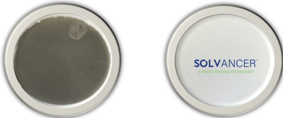
Figure 5: Impact of Solvancer on a Group II-based Air Compressor Lubricant, which lowered the varnish potential from 67 to 11. One can observe that the constituency of the deposits on this patch appear different than in Fig. 4.
