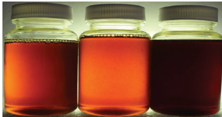
Figure 8: The color of the fluid darkened over the 3 months as part of the decontamination process as the sludge and coal dust were dissolved from the internals of the gearbox
