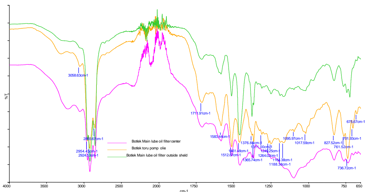
Fig. 2 FTIR Spectrum varnish fractions.
