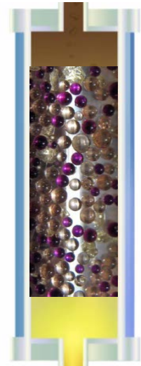
Acid levels lowered, Resistivity increased, metals and varnish molecules removed
